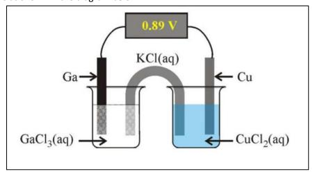
The cell potential was measured at 0.89 V, with the copper electrode gaining mass when the cell was discharging.
